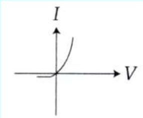
Its V-I characteristics of simple diode.
