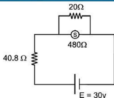
$$\text{Resistance of ammeter} = \frac{480 \times 20}{480 + 20} = 19.2 \Omega$$
