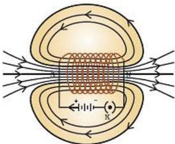
The field lines inside the solenoid are in the form of parallel straight lines. This indicates that the magnetic field is the same at all points inside the solenoid. That is, the field is uniform inside the solenoid.
