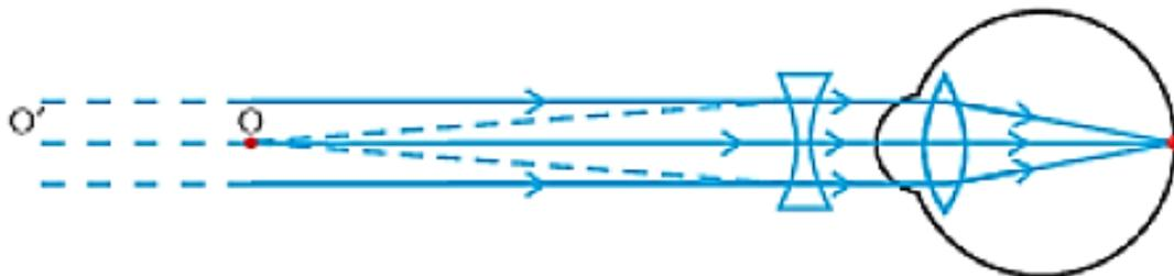
Focal length of the corrective lens used = - (Distance of far point of the myopic eye) = -1.2 m
