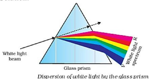
Different colours of white light bend through different angles with respect to the incident ray, as they pass through a prism. Thus the rays of each colour emerge along different paths and become distinct. It is the band of distinct colours that we see in a spectrum.
