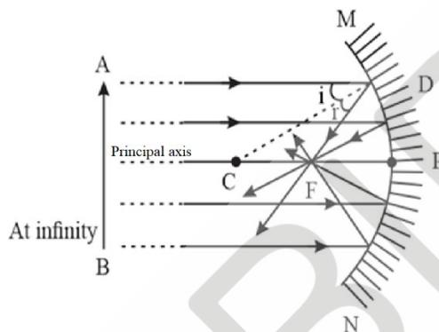
The principal focus of a concave mirror is a point (F) on its principal axis to which all the light rays which are parallel and close to the axis, converge after reflection from the concave mirror.
