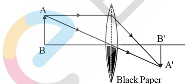
Yes, it will produce a complete image of the object, as shown in the figure above. This can be verified experimentally by observing the image of a distant object like the tree on a screen when half of the lens is covered with a black paper. However, the intensity of the brightness of the image will reduce.
