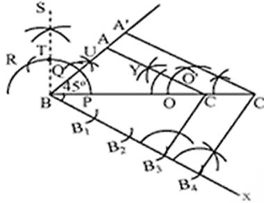
7. Draw a right triangle in which the sides (other than hypotenuse) are of lengths 4 cm and 3 cm. Then construct another triangle whose sides are  $\frac{5}{3}$  times the corresponding sides of the given triangle.
